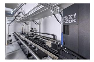
Inside view of hiXAS with X-ray source, crystal analyzer, and detector.
