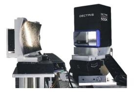
View of crystal and detector setup inside hiXAS. The HAPG crystal is specifically optimized to the target application. Extremely high resolving power and high efficiency are obtained simultaneously. The hybrid detector with large sensor area enables assessing sample homogeneity.
