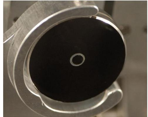
Double-mirror for pump-probe attosecond experiments. Tailored mirror coating for specific energy selection for reliable generation of isolated attosecond pulses.
