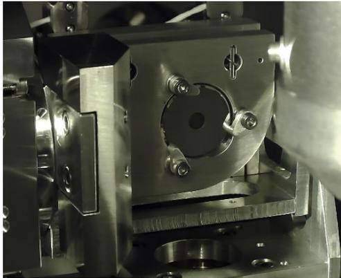
Double-mirror delay assembly XUV/VIS-IR for collinear beam refocusing. Temporal resolution of  $\pm 3\text{as}$ . 5 degrees of freedom. Spectral isolation of the cut-off region. Low wavefront distortion due to optically precise shaped segments
