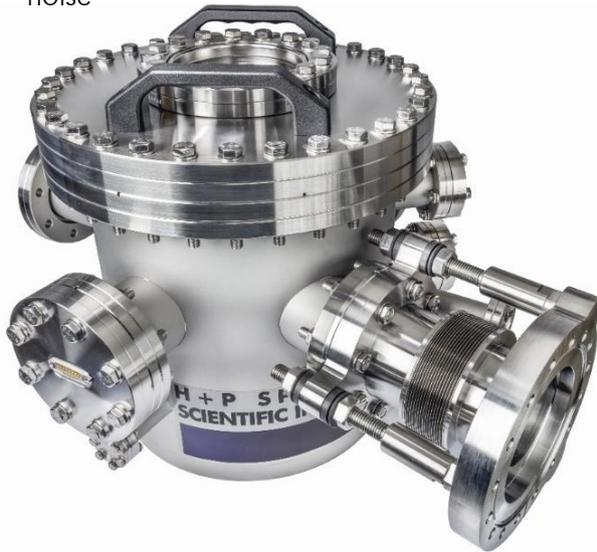
Compact spectrometer for in-situ HHG source characterization in the water window. Direct imaging of the source without entrance slit for maximum efficiency and day-to-day robustness. Undistorted beam in bypass mode. UHV vacuum setup. Longitudinal dimension <math><0.5\text{m}</math>. All settings controlled remotely by software.
