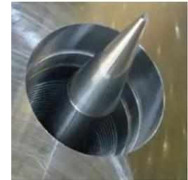
(1) Cross-drilled gas target allowing for long-term stable operation with constant gas flow. Convenient alignment with full beam due to high durability.
