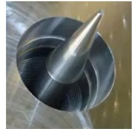
(1) Cross-drilled gas target allowing for long-term stable operation with constant gas flow. Convenient alignment with full beam due to high durability.
