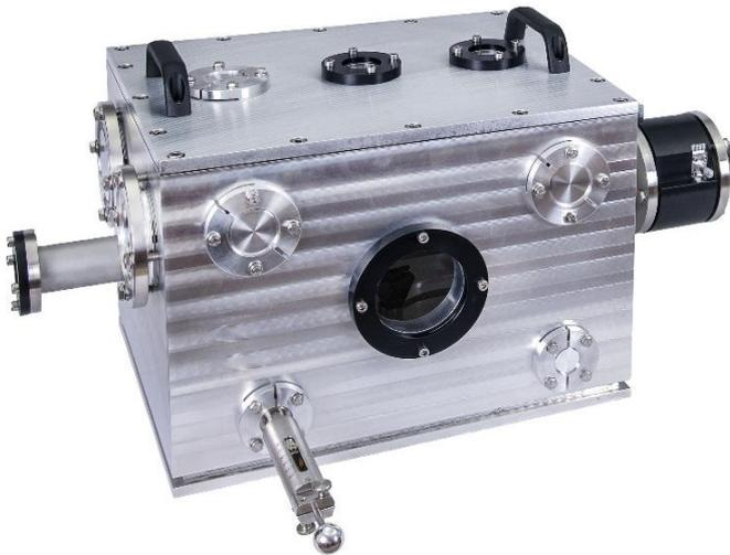
Turn-key system for investigation of high-order harmonic generation in laser-produced plasmas. Flexible motorized target setup for rotating and flat solid targets and gas targets. Multiple beam access options for two-color pumping of plasma. Integrated frequency-doubling stage. Spectral filtering stage for high-intensity beams.
