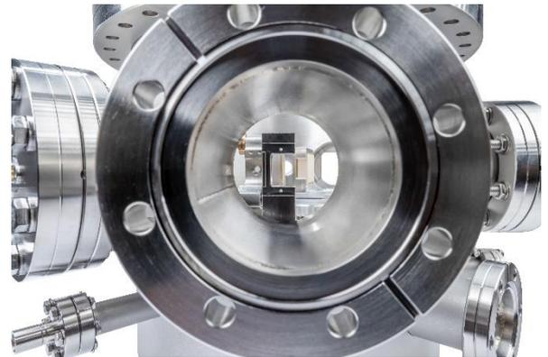
Beam-like view into in-line spectrometer. Reliable switching between bypass and spectroscopy modes by closed-loop positioners.
