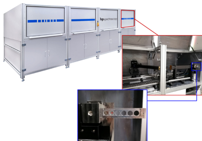
Fig. 1. Lab-XAS setup at XRAYLab, CNR ISPC (Catania, Italy); red inset: internal view illustrating the core components (X-ray source, sample holder, He-purged cells and HAPG von Hamos crystal in XANES configuration, and hybrid detector), aligned along two motorized optical rails; blue inset: a close-up of the sample holder with one position holding a small fragment of cinnabar paint.
