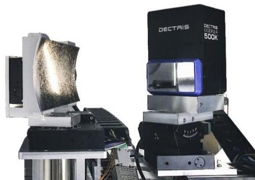
View of crystal and detector setup inside hiXAS. The HAPG crystal is specifically optimized to the target application. Extremely high resolving power and high efficiency are obtained simultaneously. The hybrid detector with large sensor area enables in-situ measurements.
